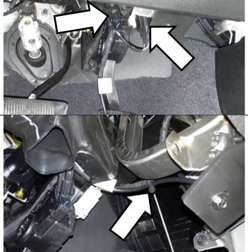
Use the supplied alcohol wipe to clean the surface where the TSBooster will mount. Apply the double-sided tape to the chosen mounting location (trim tape to length if needed).
