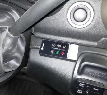
Set the desired level on the controller using the + and – buttons. See the operation section of the manual above for information on the available modes.
