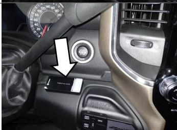
Turn the ignition switch to the on/run position but don't start the engine.
